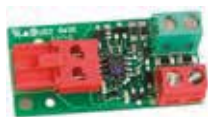
BUS XIB interface (for E045 or E024S control unit with non BUS photocell)
